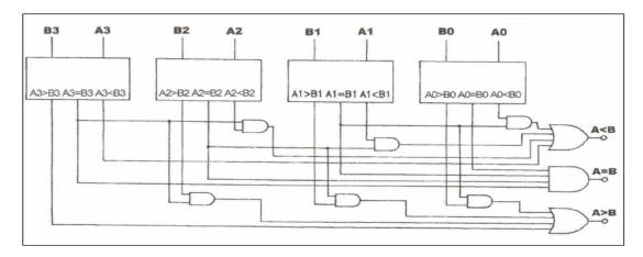
(a) Constructed with four 1-bit Comparators
