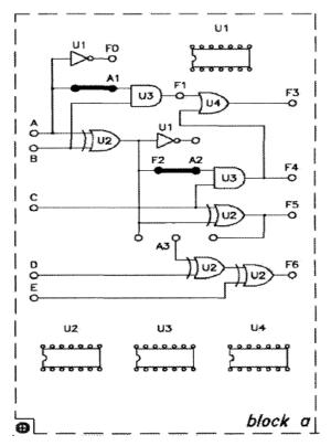
FIG1.10: Wiring Diagram (KL-26002 Block a)
