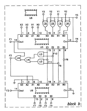
FIG1.12: Wiring Diagram (KL-26002 block b)
