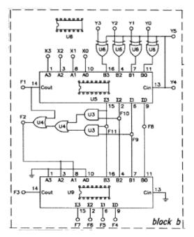
FIG1.14: Wiring Diagram (KL-26002 block b)
