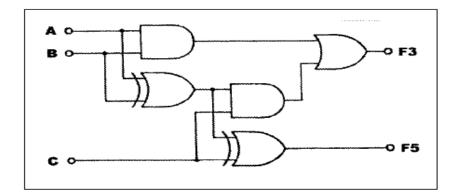
FIG1.9: Full-Adder Circuit
