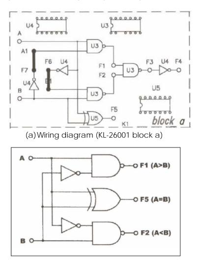
(b)Logic Diagram FIG 1.5: 1-bit comparator
