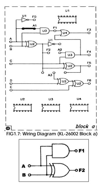
FIG1.8: Half-Adder Circuit
